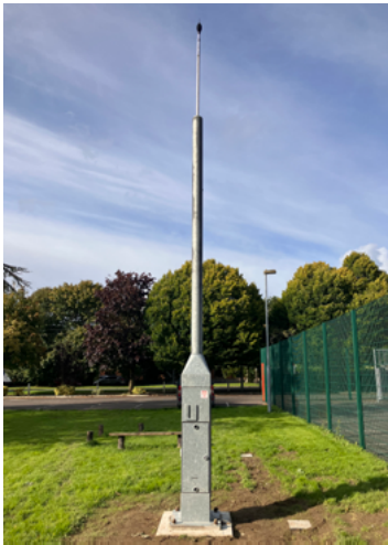
Fig. 01: A Noise Monitor Terminal (NMT) in situ
